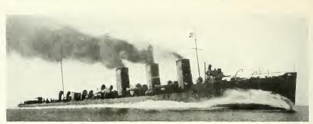
Destroyer Savifi, the fastest vessel in the British Navy: speed 39 knots.
