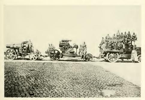
Siege gun used in the Austrian army. On the right is the motor-tractor, on the left, the gun, and in the center is the mount, which must be placed on a concrete base before the gun can be used.
