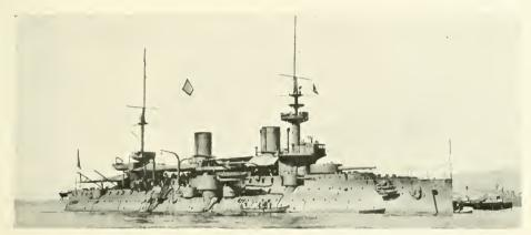
French battleship Bouvet, 12,000 tons, carrying a main armament of two 12-inch and two 10.8-inch guns.
